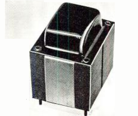
Fig. 4. Low-voltage power supply transformer shown with a copper flux shield used to reduce its 60-cycle radiation.
