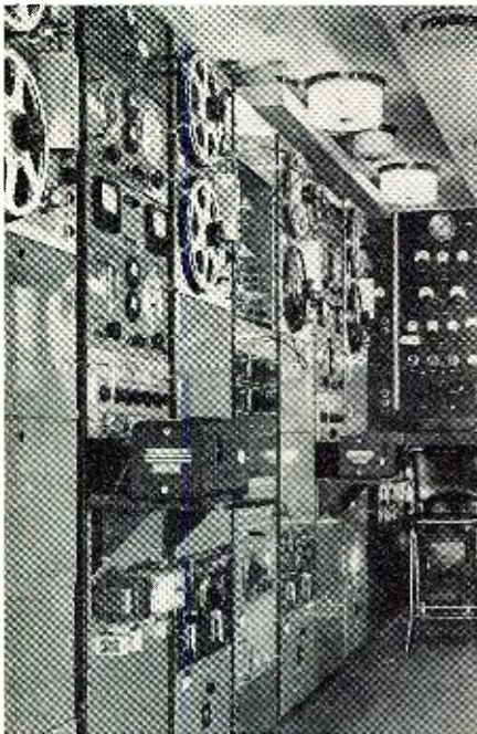
Fig. 2. The tape recorders and other equipment shown here record information transmitted to the ground station from equipment in the missile in flight.
